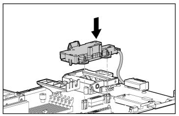
Figure 1-19: Installing the Battery-Backed Write Cache
